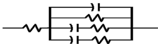
Fig. 4 Equivalent circuit to fit electrochemical impedance spectroscopic data
