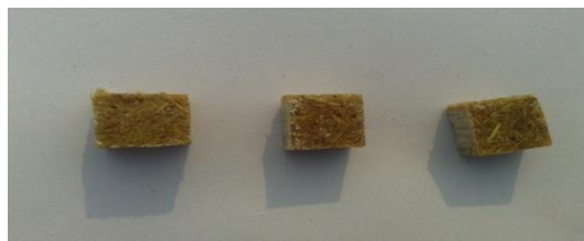
Fig. 6 Hardness test specimens as per ASTM standards
