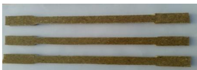
Fig. 2 Tensile Test Specimens Prepared by ASTM standards
