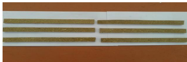
Fig. 4 Flexural test specimens as per ASTM standards
