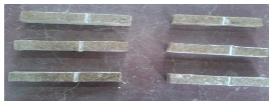
Fig. 5 Impact test specimens as per ASTM standards
